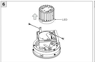
REVERSE STEPS 6-1 WHEN REINSTALLING LED INTO CEILING
