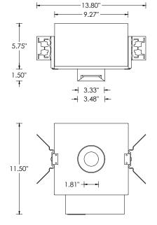
**SH -** SHALLOW HOUSING (1500LM MAX) (IC RATED AND CP RATED)
