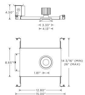
NC - NEW CONSTRUCTION HOUSING (NON-IC AND CP RATED)
