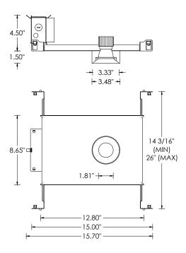
NC - NEW CONSTRUCTION HOUSING (NON-IC AND CP RATED)
