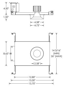
**NC-** NEW CONSTRUCTION HOUSING (NON-IC AND CP RATED) **IC -** NEW CONSTRUCTION IC HOUSING (2000LM MAX)
