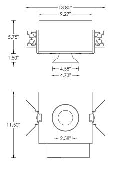
**SH -** SHALLOW HOUSING (2000LM MAX) (IC RATED AND CP RATED)
