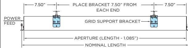
**ⓘ** APERTURE = (LENGTH - 1.085") APPLIED ONLY ON STARTER SECTION OR STANDALONE FIXTURE.
