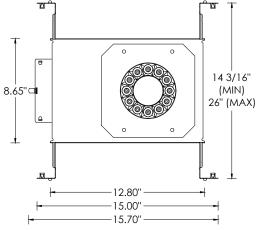
**NC-** NEW CONSTRUCTION HOUSING (NON-IC AND CP RATED) **IC -** NEW CONSTRUCTION IC HOUSING (2500LM MAX)
