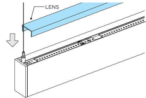
**LED SERVICING - INDIRECT - ASYMMETRIC AND WIDE SPREAD OPTIC**
