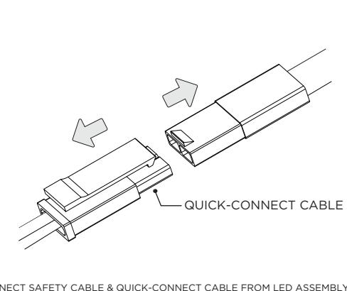
DISCONNECT SAFETY CABLE & QUICK-CONNECT CABLE FROM LED ASSEMBLY
