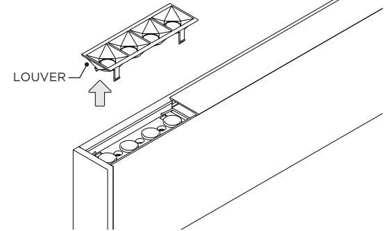
**i** REMOVE DOWNLIGHT ASSEMBLIES FROM START AND END OF ALL SECTIONS WHERE APPLICABLE
