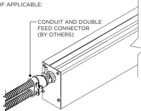
USE DOUBLE FEED CONNECTOR (BY OTHERS) FOR DUAL CIRCUIT
