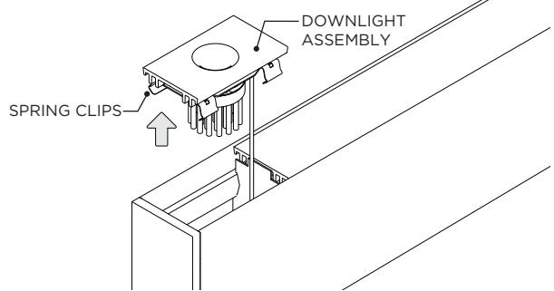
**i** REMOVE DOWNLIGHT ASSEMBLIES FROM START AND END OF ALL SECTIONS WHERE APPLICABLE
