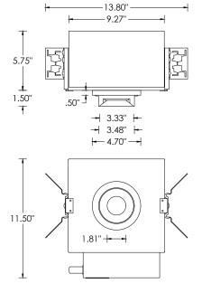
**SH -** SHALLOW HOUSING (IC AND CHICAGO PLENUM RATED) (2200LM MAX)
